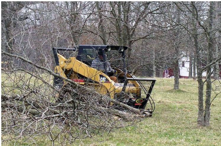
This machine, equipped with a shear (hydraulic scissors) were used to remove about 140 honey locust from the county farm.
